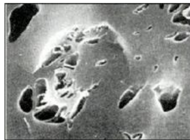
Magnified Pores in activated carbon
